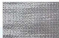
保温幕 Energy screen 遮阳率 shading rate: 15% 节能率 Energy saving: 47%
